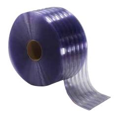
Both sides of the strip have raised ribs spaced 2" apart and are offset by 1/2" front to back. Ribbed strips are ideal for heavy traffic strip doors because they significantly reduce scratching, so the door remains clearer and safer.
