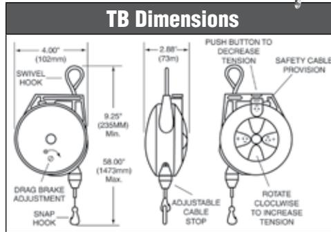
Strongly recommended, secondary steel cable or steel link chain. Prevents balancer from accidental fall. Balancers have extra holes for cable or chain.
