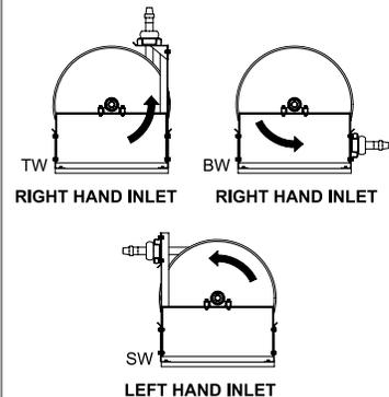
Reels are shipped in the bottom wind (BW) position. Kits are available for top wind (TW) and side wind (SW) position. Contact Reelcraft for more information.
