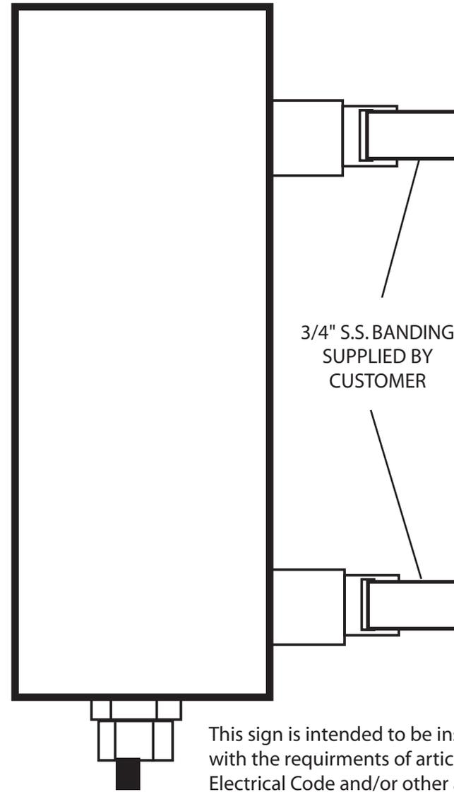
This sign is intended to be installed in accordance with the requirements of artical 600 of the National Electrical Code and/or other applicable codes. This includes proper grounding and bonding of sign"
